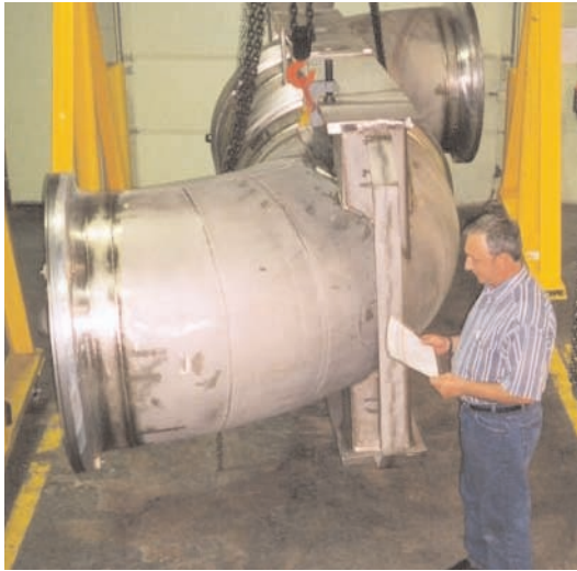
A 42" diameter TC Guide spool designed for hydrogen service
